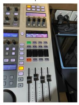
9. The main inputs to manage are the six on the left. Make sure the 'USER 1' is selected. Mute any mics not in use by pressing the relevant 'MUTE' button (which will illuminate when muted). In the example in the photo below, the 'PULPIT Left' line is in use but is muted. A
