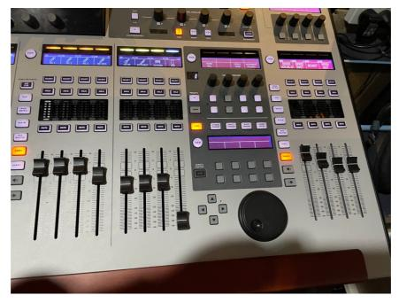
The left two of the right-most bank of four sliders are where the band channels are controlled as groups. Balance the band on the individual channels – listen on 'Solo' to work out who is on what channel - , and then adjust the overall level on the grouped faders (near the right end). Note the 'User 2' is selected for this group.
