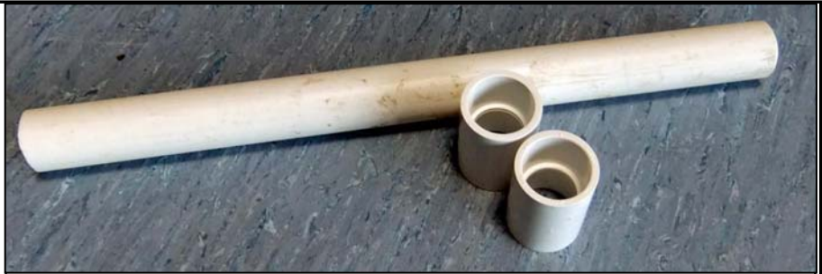
Fig 3.33 - 20mm White PVC Pressure Pipe Fittings
