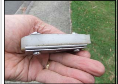
Fig 3.17 - Captive Nut for Pit Lid locking
