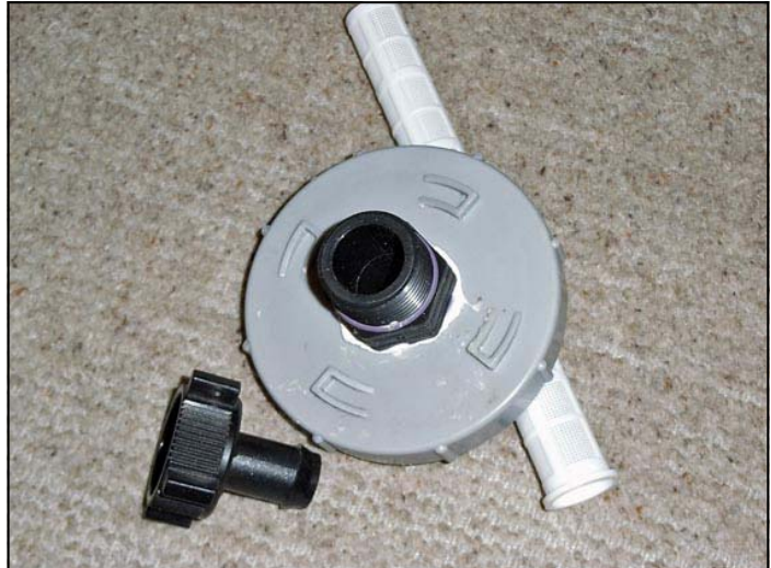
Fig 3.21 - Parts of 1st Flush Diverter
