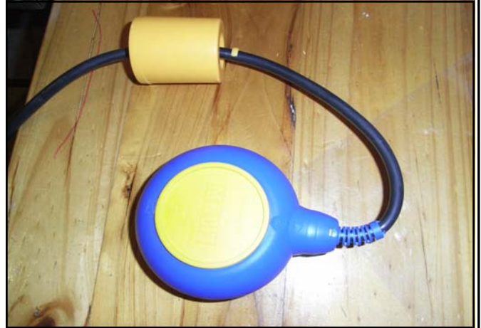
Fig 1.20 - Float level switch with weight,
