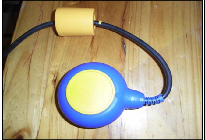
Fig 1.20 - Float level switch with weight,
