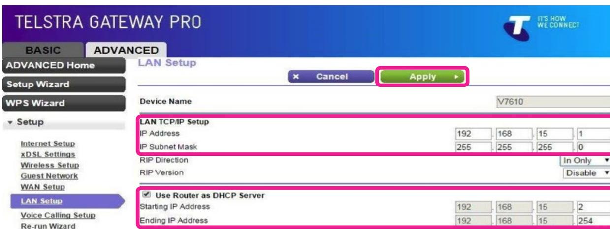
Figure 50: TCP/IP and DHCP Settings
